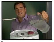
4. To accelerate condensation of the water vapour inside, pour several litres of cold water (icy if possible) over the top and sides of the drum or jerry can. Now wait until the drum implode
